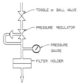
FIG. 1 Apparatus for Measuring the Silt Density Index
